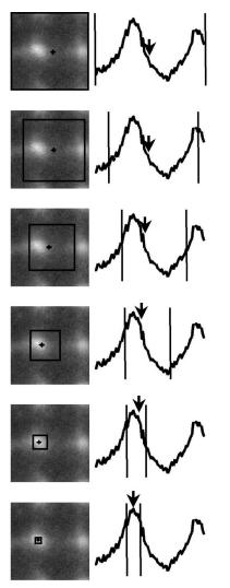
Fig. 3. Illustration of the centroiding algorithm. The top panel shows the centroiding error that would be obtained with a simple algorithm that determines spot centroids by computing the center of mass within each search box. Successive panels show the result of the new algorithm after each iteration, until finally in the bottom panel the spot centroid is accurately determined.
