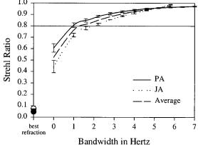
Fig. 11. Time-averaged Strehl ratio versus bandwidth for a perfect adaptive optics system, calculated for 4.7- and 5.8-mm pupils for paralyzed accommodation and for natural accommodation on a far target. Error bars on each subject's curve represent the standard deviations of the calculated results for that subject. Values of Strehl ratio higher than 0.8 are considered to correspond to diffractionlimited imaging.
